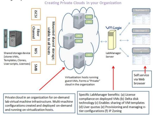
In the figure, users connect to LabManager server which manages a set of virtualization hosts using a web browser. The virtualization hosts are
